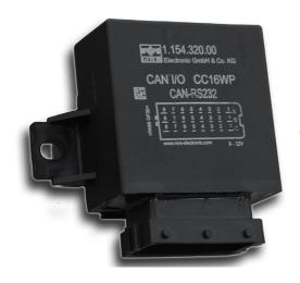
Powerful and robust control module for evaluating connected sensors and controlling various outputs. ENSIO software runs on this module to perform various functions more quickly (centering, row buttons).
